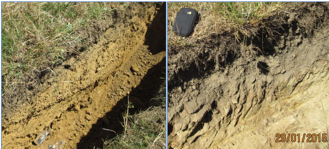
Figure 1 Typical soil profile from TP4 - topsoil over gravelly CLAY (left) and TP2 - topsoil over clayey GRAVEL grading to weathered ROCK (right).
